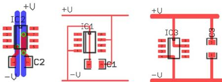
28. In the diagram of any electronic circuit, we find a number of capacitors of values typically 1 nF to 100 nF connected between the supply voltage and ground. It is also often stated that they must be placed close to the integrated circuit. What are they called and what is their function?
