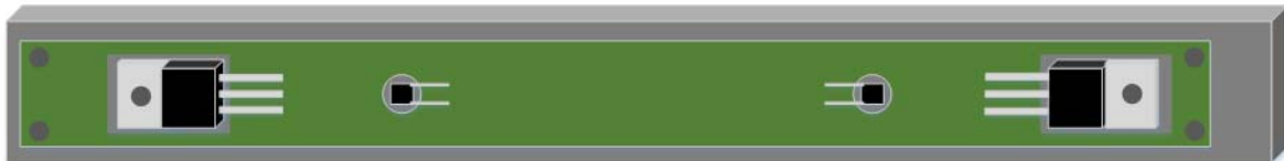
Figure 8: Heater board mounted on side Al block
